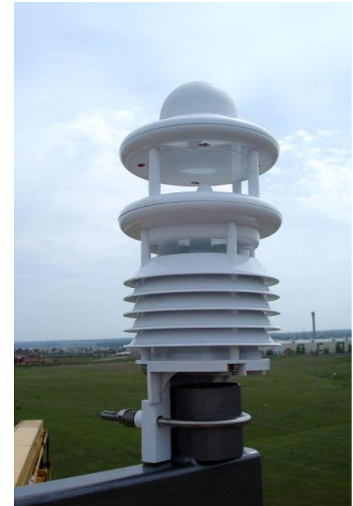
The Lufft WS-600 Weather station
